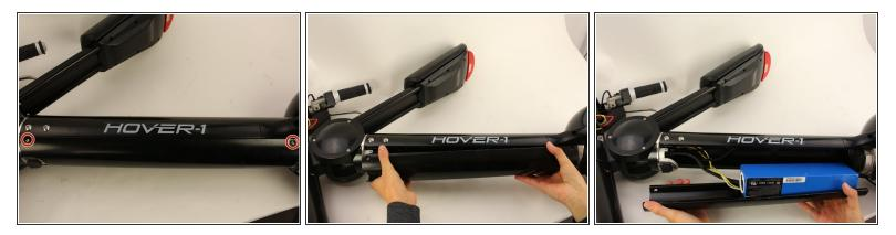
• Remove the four, 12mm Hex #3 screws located on the bottom half of the battery compartment.
