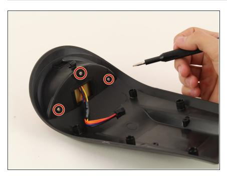
Use a Phillips #2 screwdriver to remove the four 10mm screws on the bottom of the back seat.
