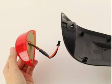
• Pull the light from behind the bottom of the seat frame. Pull the wiring all the way through.
