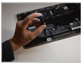
Remove the four 5mm Phillips #00 screws that hold the battery in place.
