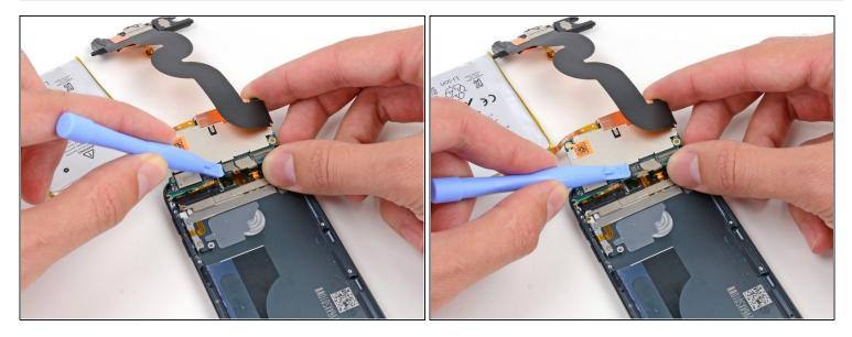
• Disconnect the button ribbon cable connector from the back of the logic board.
