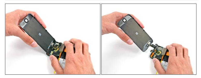
• Remove the display assembly from the iPod.
