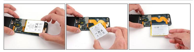
• Once all of the adhesive is loosened, lift the battery up from the bottom and swing it out over the left side of the rear case.
