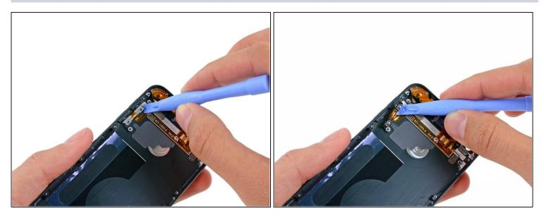
• Use a plastic opening tool to pry the left end of the button ribbon cable away from the side of the rear case.
