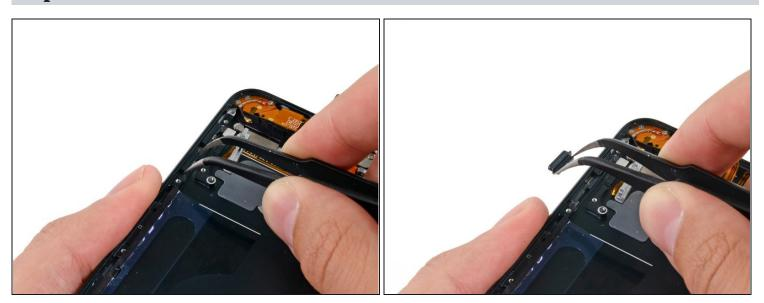
• Use <u>tweezers</u> to remove the volume-down button from the iPod.
