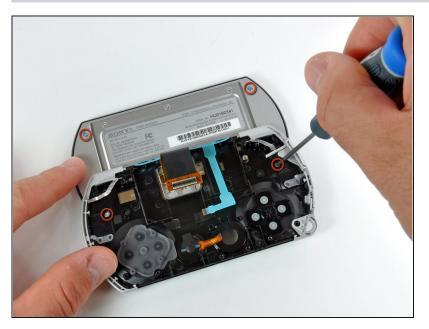
Use a #00 Phillips screwdriver to remove the four display screws.
