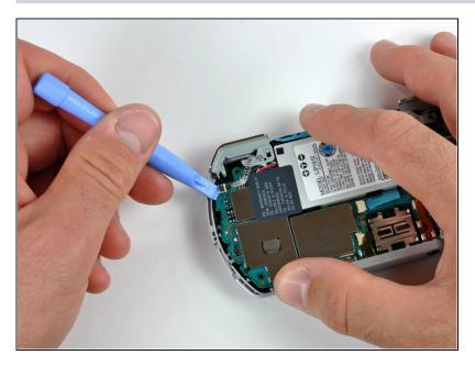
• Use a plastic opening tool to gently flip up the left trigger connector.
