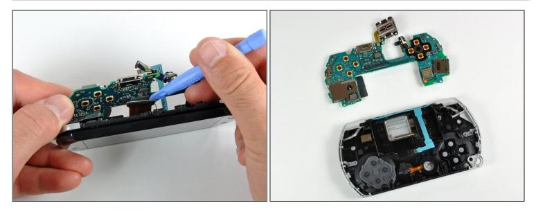
• Use a plastic opening tool to disconnect the display cable from the logic board.
