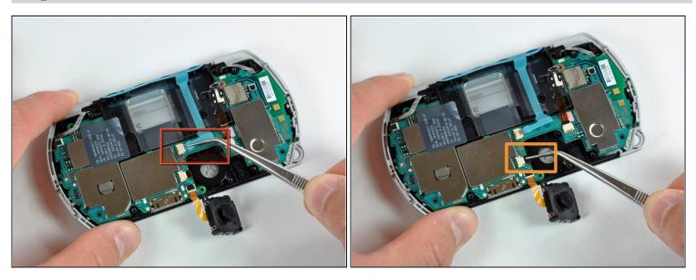
A Be very careful when disconnecting the following cables. The connectors do not have flip-up tabs; just hold each cable steady and pull it out of the connector.
