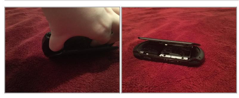
• using your thumb and pointer finder, get the 2 top ends of the UMD holder and pinch together, you've done this correctly if the trays close to the door.
