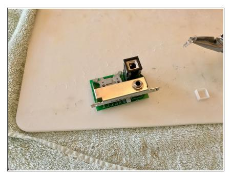
• Be careful and remove old bulb with needle-nose pliers.
