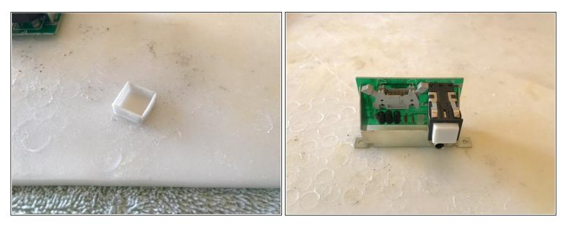
• The cover will have two small holes and two larger notches. The two smaller notches will go up and down and the larger notches go left and right.
