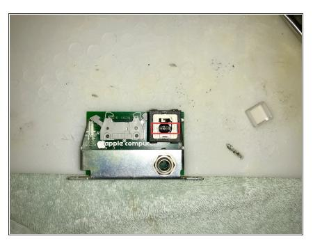
• When inserting the new bulb be careful to line up the prongs.
