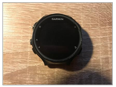
The strapless 735xt, the straps are secured by two T6 screws on each side.
