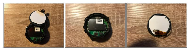
• Once the screen moves, carefully remove the ribbon connector and the screen.
