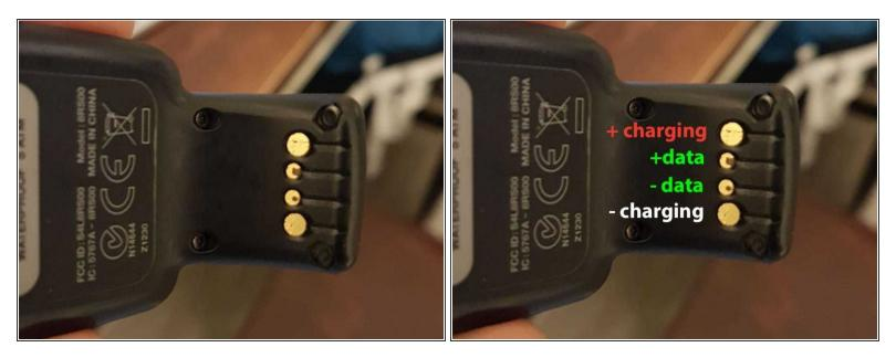
Inspecting the back we can see some pin pads are not 100% functional
