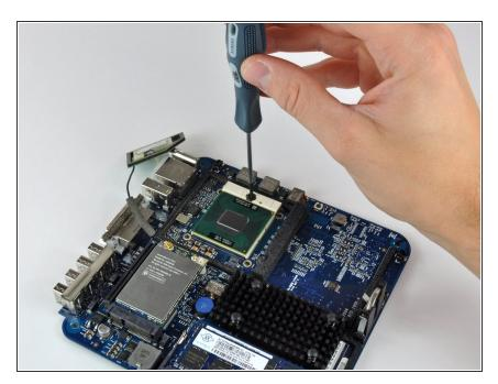
Use a small flathead screwdriver to rotate the processor lock 180 degrees clockwise until the indicator points toward the closed lock symbol.
