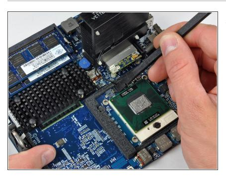
Lay the heat sink on the AirPort card and use a spudger to reconnect the heat sink thermal sensor.
