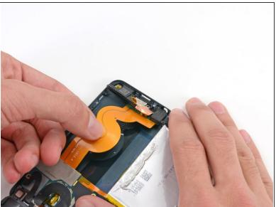
Grasping the large ribbon cable, gently pull the Lightning connector assembly out of the bottom of the case.
