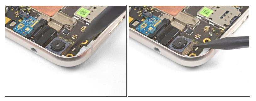
Use the point of a spudger to pry up and loosen the front facing camera module. from its socket.
