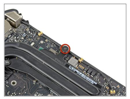
Remove the single 5 mm T6 Torx standoff from the heat sink near the edge of the logic board.
