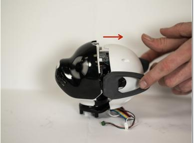
Remove the 4 Phillips screws on back of the head, and pull off the casing for the back of the head.
