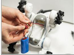
Once the battery is removed from body, the battery should be connected by a red and black wire.
