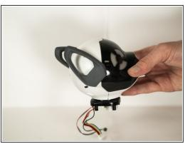
Remove the 4 Phillips screws to separate the head from the body.
