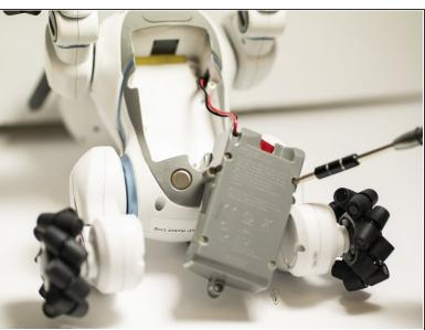
Once the top face of the battery is off, you will see a small rectangular box that the batteries are inside. There are 4 Phillips head screws in the box. Remove all screws with a Phillips head screwdriver.
