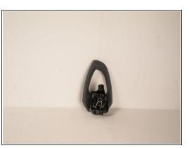
Unscrew the screw on the ear with a Phillips screwdriver, and pull off the plastic connector.
