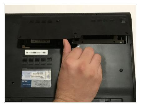
Lift backplate and remove from the case.
