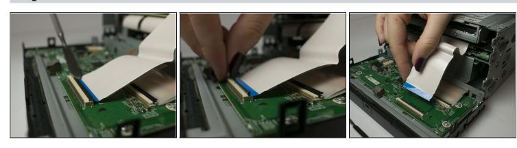
Gently separate the ribbon cable from from ZIF connector on the circuit board using a metal smudger.
