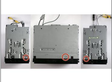
• Remove three steel-finish, pan-head, 1/64 x 3/16" machine screws identified in the photograph, using the Phillips #0 screwdriver.
