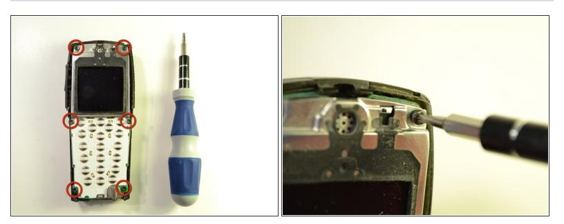
• Remove the six screws highlighted by the markers using the screwdriver.
