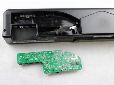
Disconnect the cords running to the white connecter by pulling up on the tab until it is disconnected completely.
