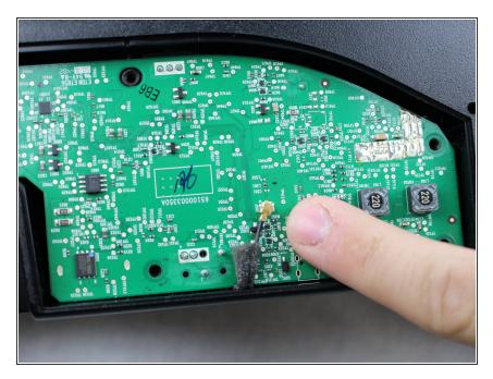
Remove the gold plates snap connector from the circuit board by pulling it apart.
