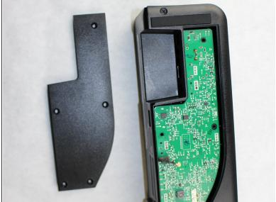
Remove the five 18.25mm screws with the Phillips #2 screw driver.
