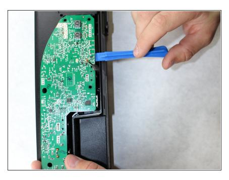
Using the plastic opening tool, lift the circuit board up and remove from housing.
