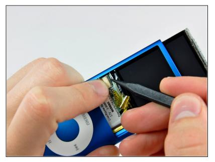
• While holding the light colored socket down with one finger, use the tip of a spudger to flip the ZIF cable lock up toward the bottom of the Nano.
