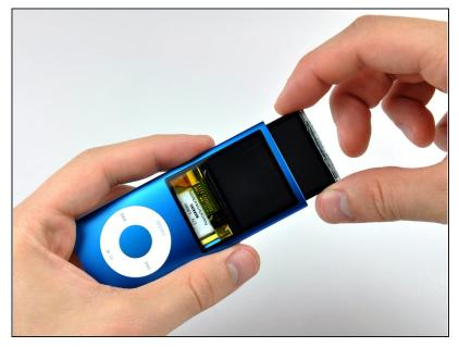
Slide the display out of the Nano. It will move about .5" until the display data cable limits its travel.
