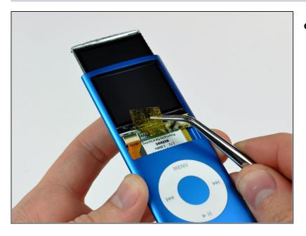
• Peel back the Kapton tape covering the display data cable socket.
