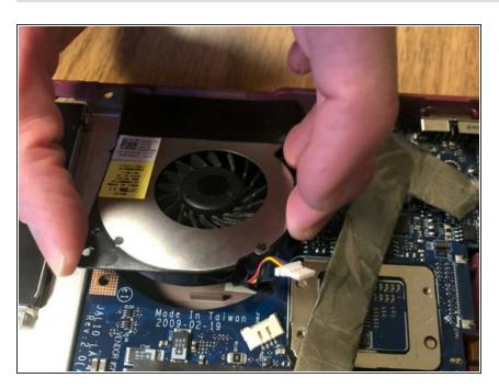
Lift the fan upwards and remove it from the device.
