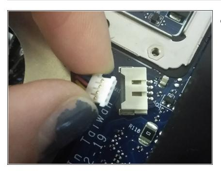
Disconnect the wires that connect the fan to the rest of the computer.
