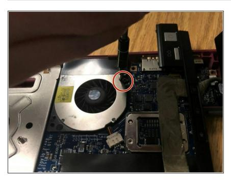
Using a Phillips 1 Screwdriver, remove the two M2.5x5-mm screws located on opposite sides of the fan.
