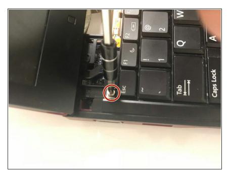
Using a Phillips 1 Screwdriver, unscrew the three M2x3-mm screws located above the keyboard where the small panel was originally.
