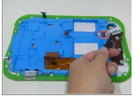
Once the blue ribbon cable is disconnected from the motherboard, use tweezers to carefully pull the ribbon cable out of the slots.
