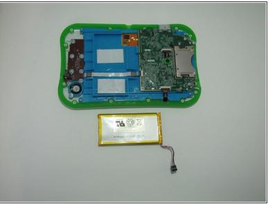
Carefully remove the battery from the LeapPad. Use an opening tool or a plastic spudger to gain leverage, if needed.
