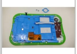
Remove the circular plastic speaker and the 2 screws a Phillips #1 screwdriver. Gently lift the cover off of the device.
