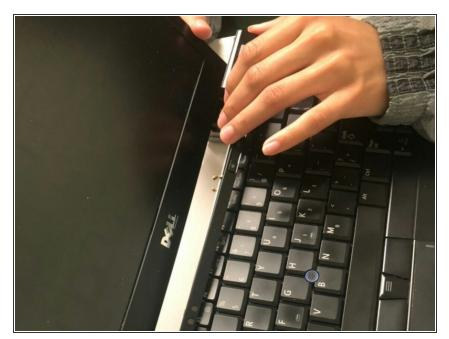
Open the laptop and remove the small panel located above the keyboard.
