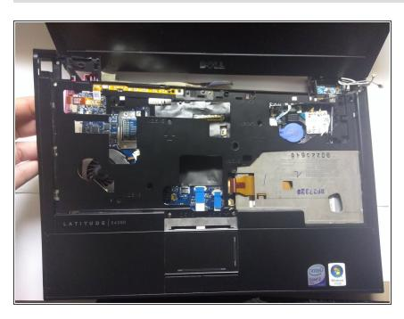
Lift the keyboard panel to separate the component from the rest of the device. To reassemble your device, follow these instructions in reverse order.
