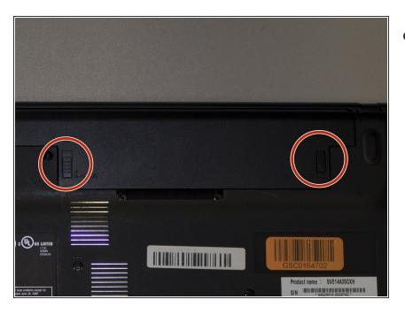
Locate the lock and release switches on the battery.
