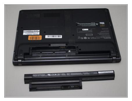
Finally, remove the battery pack from the computer.
