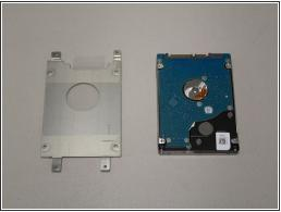
Remove the four screws holding the hard drive bracket to the hard drive using a Phillips #0 screwdriver.
