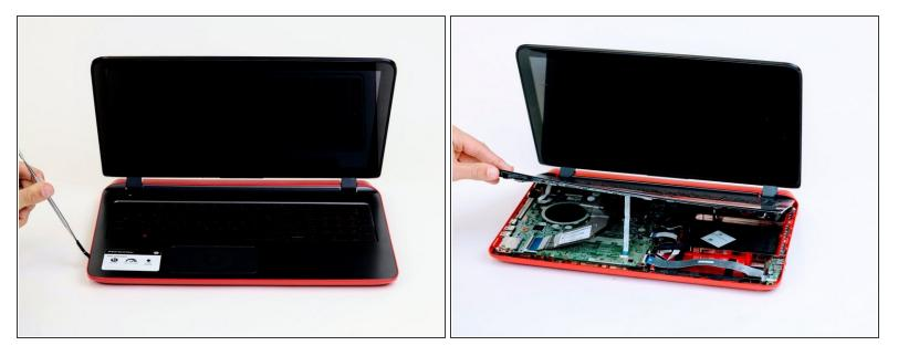
• Flip computer over and wedge metal spudger along the computer to pop off keyboard panel
