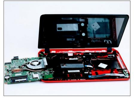
• Detach by lifting the motherboard up and flip the motherboard over.
