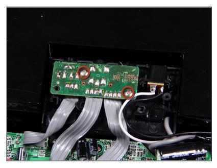
• Remove the two 10 mm Phillips #0 screws attaching the circuit board to the case.
