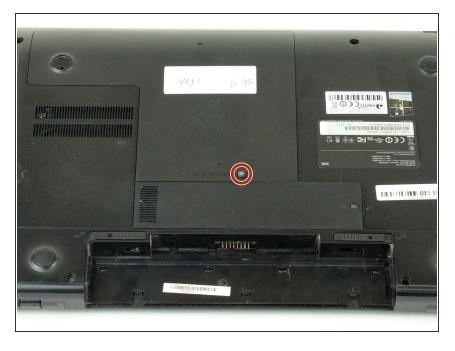
Remove the M2.5x5 mm screw with a Phillips #0 screwdriver.
