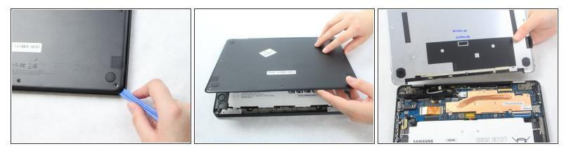
• Slide the plastic opening tool in a corner at a steep angle, and lift up to remove the outer case.
