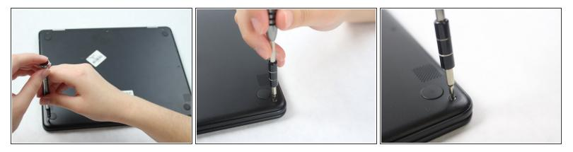
• Remove the eight 30 mm screws from the edges of the case with the JIS J000 screw bit.
