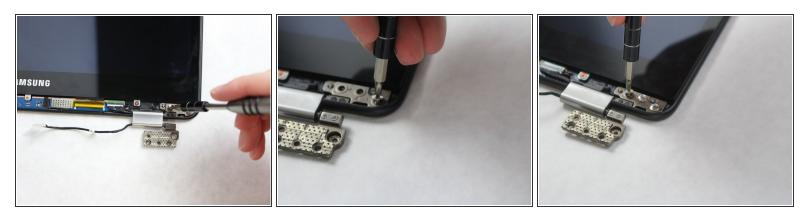
• Remove the three 30 mm screws from hinge plate R1 and L1 using the JIS J000 screw bit.
