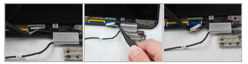
• Disconnect the black wire on the R1 plate connected to the screen using the precision tweezers.
