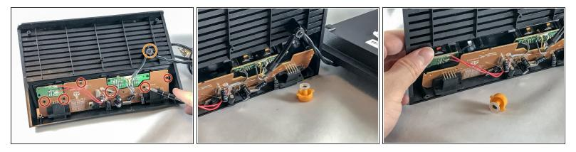
Unscrew the six 9.0 mm Phillips #1 screws on the brown circuit board that correspond to the reset and select buttons.
