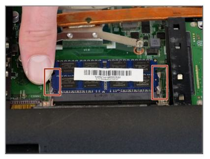
Press the tabs on the side of the RAM to remove it.
