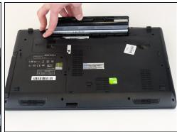
Slide and hold the release tab on the left side of the battery, so that you can remove the battery.
