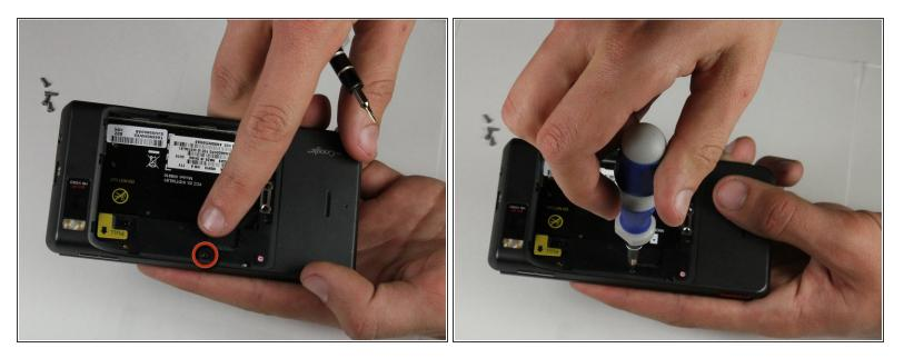
Flip the phone over and locate the screw on the middle of the left side. Unscrew it using the T5 Torx screwdriver and set it aside.
