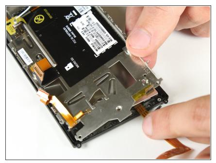
• Carefully separate the metal plate from the LCD and front housing.
