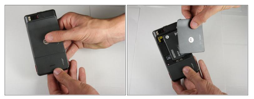
• Place thumb on the back cover, and push down towards the bottom of the device. Once the cover releases, pull it away from the phone and set it aside.
