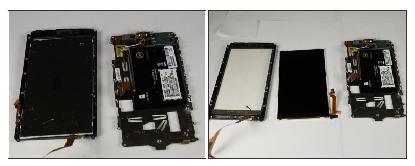
• Lift the LCD out of the front housing.
