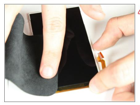
Remove all dust and smudges from the LCD and front housing before installing the screen.
