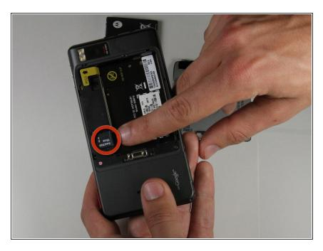
• Remove the micro SD card from its connector.
