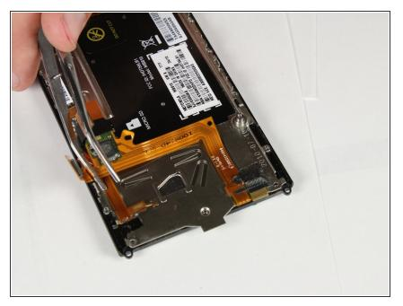
Using tweezers, peel the orange and black cable away from the device, stopping before reaching the electrical tape at the near the edge of the screen.
