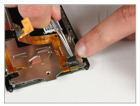
• Peel black the black electrical tape located near the bottom of the device.
