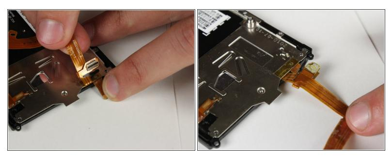
$\bigwedge$  Carefully pull the long orange cable away from the device.
