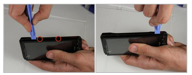
Locate the seam along the right edge of the phone. Use the prying tool to disconnect the two clips along the edge.
