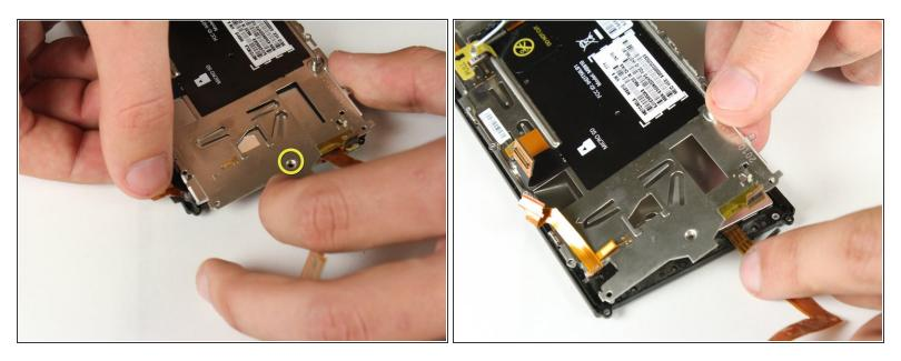
• Unscrew the screw at the base of the screen using the T4 torx screwdriver .
