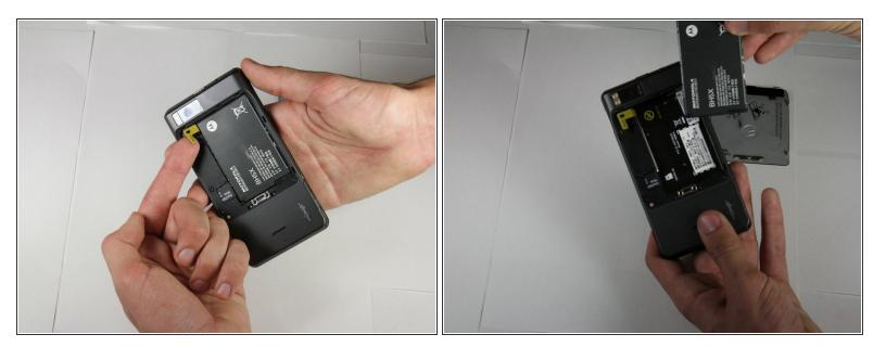
• Find the yellow pull tab located in the upper left corner. Pull the tab until the battery dislodges. Grab the battery by the raised edge, and remove it from the case.
