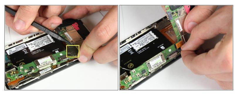
Scrape away the electrical tape that covers the LCD and digitizer cable using the spudger tool or a fingernail.
