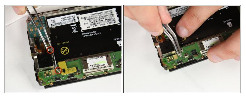
• Carefully remove the white connecting wire from the motherboard using tweezers.
