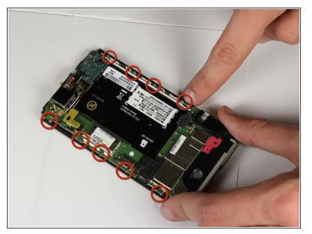
Remove the screws along both sides of the motherboard using a T3 Torx screwdriver. On some phones this may require a #1 Phillips Screw Driver.
