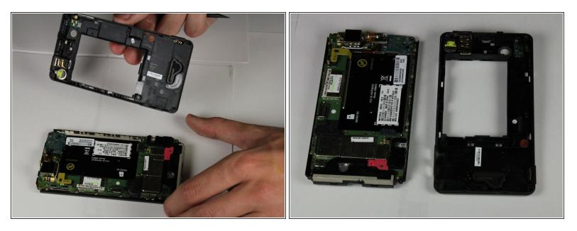
• After the clips are detached, remove the back case and set it aside.
