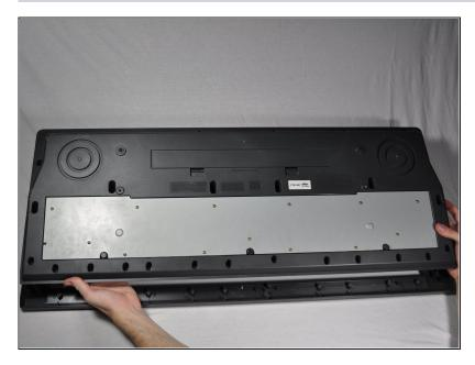
• Remove the bottom panel by lifting and pulling it towards yourself.
