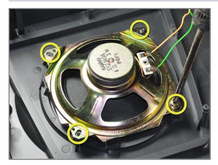
• Completely screw in the screws back into the original positions on the corner of the speaker.
