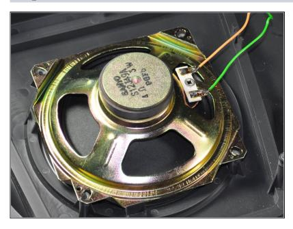
• Pull the speaker out of the keyboard and set on a flat surface to solder safely.
