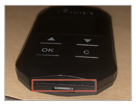
Place spudger or small flathead screwdriver into the gap on the bottom. Carefully move around the case and unclip the plastic.
