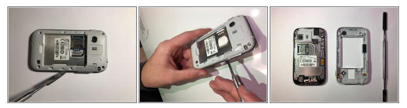
• Use the metal pry tool to separate the interior back panel from the interior hardware and screen.
