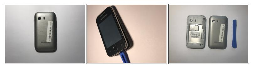
• Use the blue plastic opening tool to pry the back-panel off of the device.
