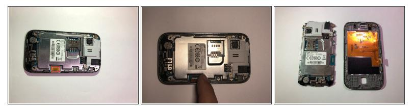
Disconnect the orange motherboard connection, then remove the interior hardware from the front screen display.
