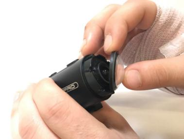
Remove the blue securing the lens cover. Then simply pull off the lens cover itself.
