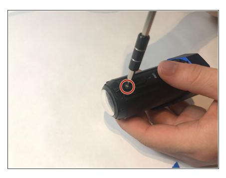
Using a #00 Phillips screwdriver, unscrew the screw securing the record/stop switch.
