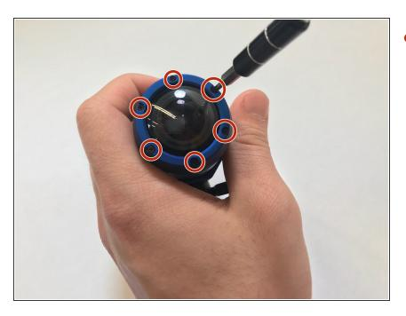
Remove the six screws (3 mm) that secure the lens cover bezel with a #00 Phillips screwdriver.
