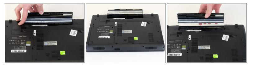
• While holding the release tab, remove the battery slowly.
