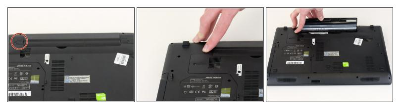
Slide and hold the release tab on the left side of the battery, so that you can remove the battery.
