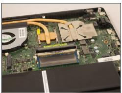
Push both metal tabs away from each other on each side of the RAM farthest from battery so that the RAM will pop up.
