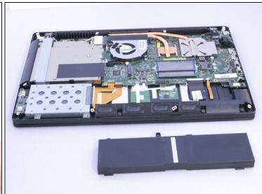
Once the screws have been removed, gently lift the battery out.
