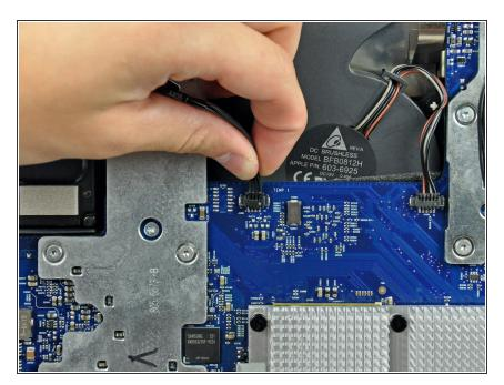
Disconnect the hard drive thermal sensor from the logic board by pulling its connector toward the top edge of your iMac.
