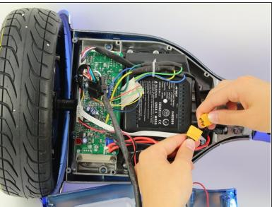
Disconnect the battery by holding the yellow connectors and pulling apart.
