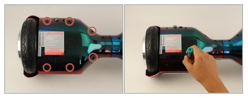
• Remove the six 12mm Phillips #2 screws holding the base plate.
