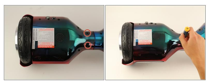
• Remove the two 11mm Phillips #1 screws that hold the base plate to the body.
