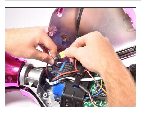
Lift the shell without the speaker grille and unplug the battery.
