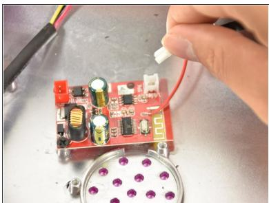
Disconnect the cable attaching the speaker to the sound card.
