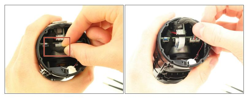
Pull the wire coated with dark gray foam out from the space where it is tucked and move it out of the way.
