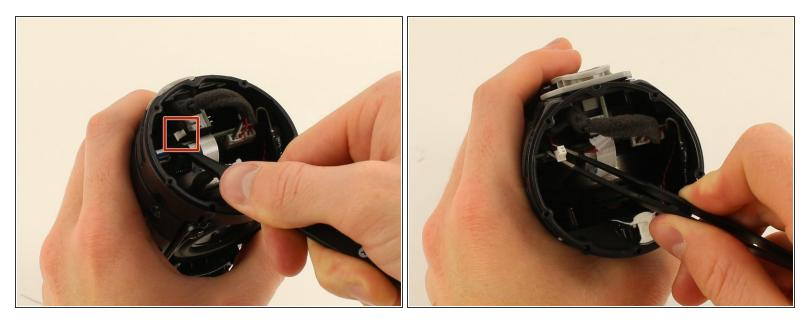
Unhook the other smaller white plug behind the previous plug from the same small hanging circuit board using the tweezers.
