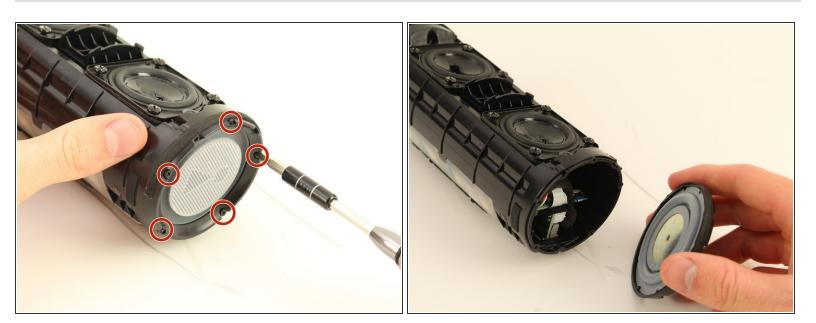
• Remove the five 9mm Phillips #1 screws to remove the endcap.
