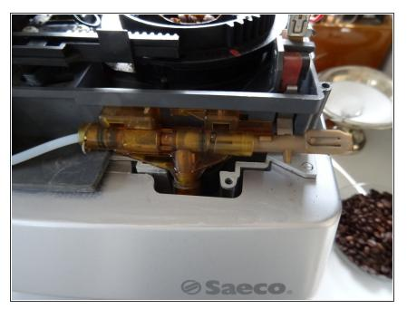
The steam valve is located on the top right of the machine. If it has cracks, water will drip out of the valve body.
