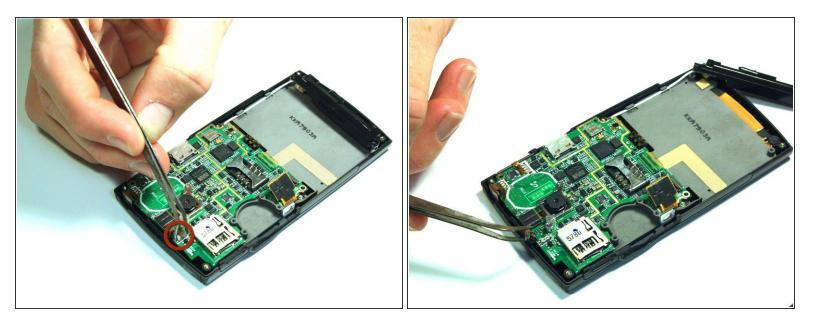
Use the tweezers to unsnap the connection between the motherboard and the speaker. The speaker is attached to the front casing.
