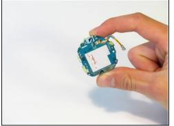
Remove the battery's cable from the chassis using tweezers.
