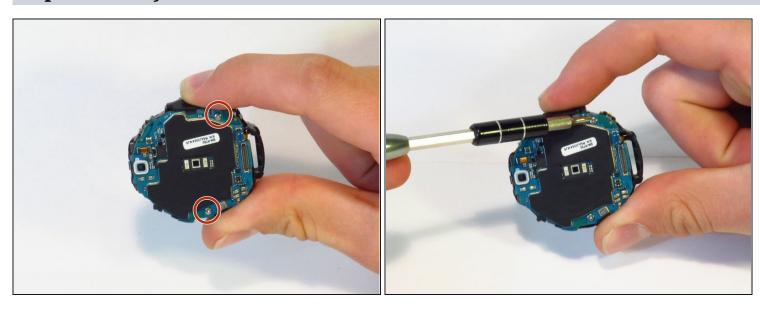
• Using a JIS #00 screwdriver, remove the two 4.5 mm screws.
