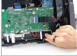
Remove the the black cable from the bottom of the motherboard by carefully pulling down on the connection.
