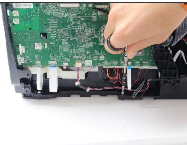
Remove the two 9.3 mm T9 screws that attach the power supply to the bottom of the printer.
