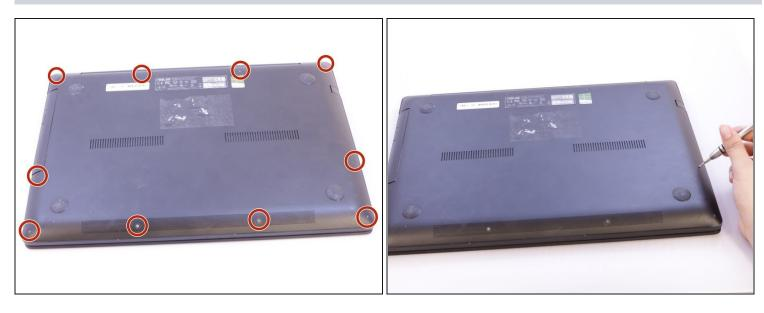
Use a T4 Torx screwdriver head to remove the ten 4mm Torx head screws on the bottom of the laptop.
