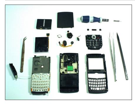
• From top to bottom, left to right: battery, back cover, screw handle, PH00 screw bit, small tweezers, camera screen, antenna cover, antenna and speaker, volume dial, speaker, power button, volume, button, back button, keypad cover, tweezers, spudger, logic board, back case, front case
