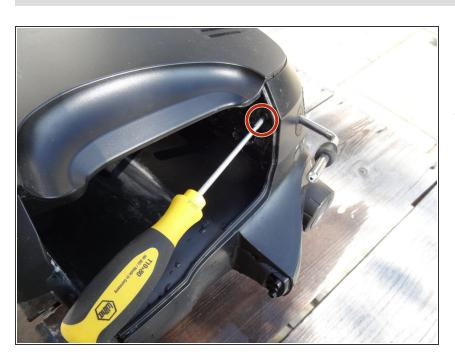
Place the machine on its side. At the bottom of the top cover, to the left and right of the coffee spout, are two Torx T10 screws. Remove those.
