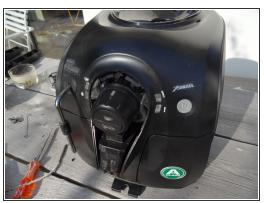
The cover over the coffee spout is held by detents. To release those insert a plastic opening tool.
